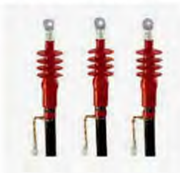
ABOVE PHOTO SHOWS THE INDIVIDUAL XLPE CABLE TERMINATION ON A THREE PHASE CABLE TERMINATIONS FOR TAKE-OFF STRUCTURE APPLICATION. EITHER 3M COLD SHRINK TYPE OR HEAT SHRINK TYPE BY RAYCHEM CABLE TERMINATIONS RATED 15kV CLASS.
